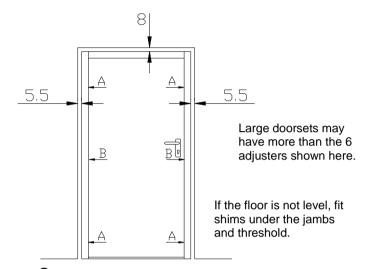
2. Align and grip the doorset in the opening, using the frame adjusting screws A in the corners, then the middle adjusters B.
