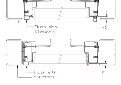
**5.** Set the lock jamb flush, as shown above, or set back from the outer steelwork.
