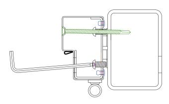
**9.** Open the door fully, then tighten the frame adjusters in the reveals.
